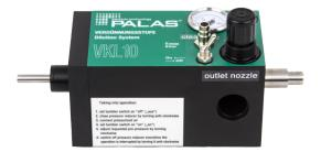
The VKL 10 series of dilution systems can reduce the concentration of aerosols by the dilution factor 01:10, also of very highly concentrated aerosols, in a defined and reliable way.
