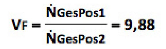
Provided the first measurement is not affected by a coincidence error and the dilution system under test is working (not soiled), a dilution factor of almost 10 is determined. If this should not be the case, there was possibly a coincidence in measurement 1. In this case, the aerosol concentration has to be decreased or a further dilution step used. Another possibility would be that the dilution step to be tested is soiled. In this case, the device has to be cleaned and the test repeated.
