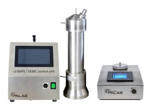
A soft X-ray source as a neutralizer is already integrated. The advantage instead of a radioactive neutralization (for example, with Kr-85) is that there is no need to follow requirements during transportation.
