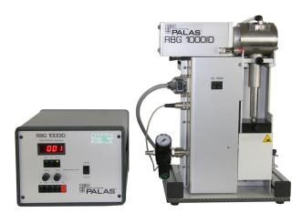
This device disperses particles at positive pressure values of up to 3 bar and can also use nitrogen, in addition to air, as the dispersing gas.
