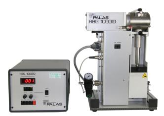
This device disperses particles at positive pressure values of up to 3 bar and can also use nitrogen and air as the dispersing gas.
