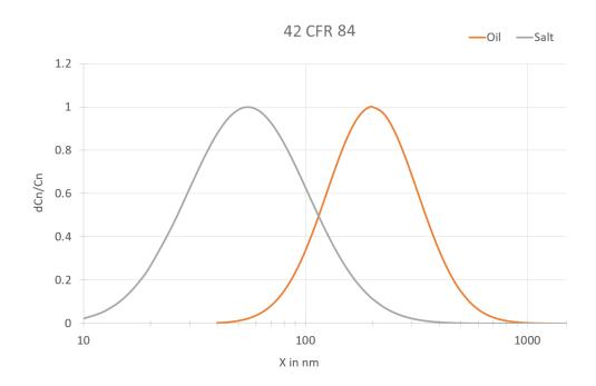
Based on the measurement of the particle penetration via the particle size, the PMFT 1000 F can also be used to consider the tolerances in the particle size distribution according to EN 13274-7 as min. / max. penetration value.
