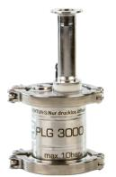
The PLG 3000is used for fractional separation efficiency measurement and loading with oil aerosols as per ISO 12500-1. The oil quantity can be adjusted using the dispensing volume flow between approx. 0.2 - 12 g/h. The PLG 3000 aerosol generator is designed to be pressure-resistant up to 7 bar positive pressure (higher pressure values upon request).
