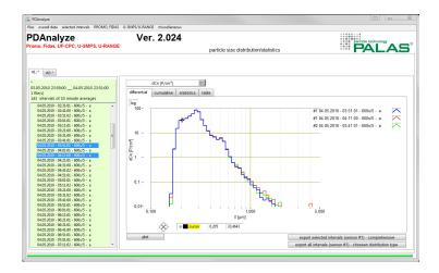
The PDAnalyze software is designed to acquire measurement values and data analysis by all stand-alone particle measuring devices. It enables quick and easy analysis of particle sizes and concentrations using the Promo® System, Fidas® System, UF-CPC System, U-SMPS System, and U-RANGE System.
