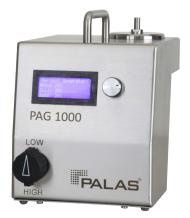
The autonomous PAG 1000 (Portable Aerosol Generator) offers maximum flexibility for generating droplet aerosols, for example, from DEHS or low-concentration salt solutions.
