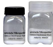
MP 40 are microparticles with a mean diameter of 40,06  $\mu$ m. The distribution of this dust is monodisperse; the geometric standard deviation of the distribution is only 3,56  $\mu$ m. Due to this small distribution, these dusts are used for scientific analysis and can also be used to calibrate measuring devices.
