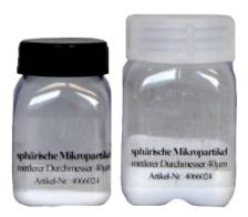
MP 20 are microparticles with a mean diameter of 20.56  $\mu$ m. The distribution of this dust is monodisperse; the geometric standard deviation of the distribution is only 4.56  $\mu$ m. Due to this small distribution, these dusts are used for scientific analysis and can also be used to calibrate measuring devices.
