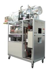
With the MFP 3000 HF, it is possible to set the relative humidity from 10 to 80 % or the temperature from -10 to 50  $^{\circ}$ C. The inflow velocity has been extended compared to standard models to a range of 4 cm/s – 2 m/s.
