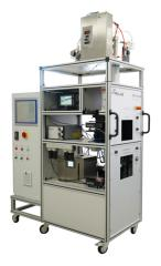
Version MFP 3000 G is especially tailored to the requirements of the ISO 16890 measurement procedure.
