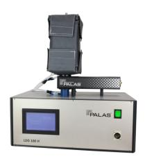
The dilution of large droplets is significant when measuring highly concentrated droplet aerosols. Since large droplets are challenging to dilute, standard systems only work up to a size of 1 - 2  $\mu$ m. The model variant LDD 100 H can be heated up to 150 °C and thus prevents condensation.
