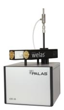
The dilution of large droplets is significant when measuring highly concentrated droplet aerosols. Since large droplets are challenging to dilute, standard systems only work up to a size of 1 - 2  $\mu$ m. The dilution system LDD 10 (dilution factor 10) is the first system to dilute almost loss-free large droplets up to  $10~\mu m$
