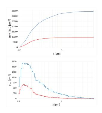
Analysis in table form, including the test conditions Example: Fractional separation efficiency measurement on the MFP 2000
