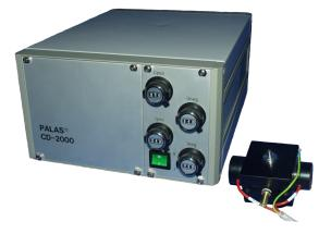
The CD 2000 type B bipolar discharge unit uses a mixed airflow of  $3 - 36 \text{ m}^3/\text{h}$  with a tube diameter on the aerosol inlet of  $\emptyset i= 13 \text{ mm}$ .
