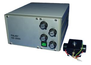
The CD 2000 type A bipolar discharge unit uses a mixed airflow of  $2 - 18 \text{ m}^3/\text{h}$  with a tube diameter on the aerosol inlet of  $\emptyset$ i= 6 mm and  $\emptyset$ a= 8 mm.
