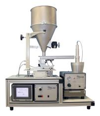
This dispersion system can continuously generate the highest mass flows, e.g., 7.3 kg/h, with the highest dosing constancy and control with automatic mass flow monitoring. The automatic refill and weighing units enable this dispersion system to be successfully used for continuous dosing over several days. Mass flow setting of approx. 350 g/h - 7.3 kg/h based on SAE fine, A2 dust.
