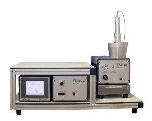
This dispersion system is able to generate high mass flows continuously, e.g., 7.3 kg/h, with optimal dosing constancy and control with automatic mass flow monitoring. Mass flow setting of approx. 350 g/h - 7.3 kg/h based on SAE fine, A2 dust.
