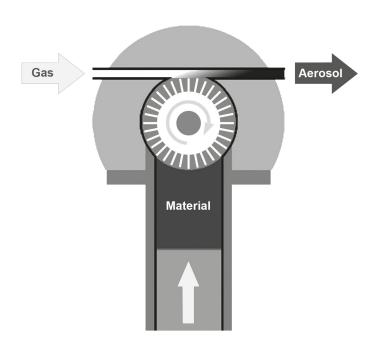
Fig. 1: Schematic diagram of RBG system
