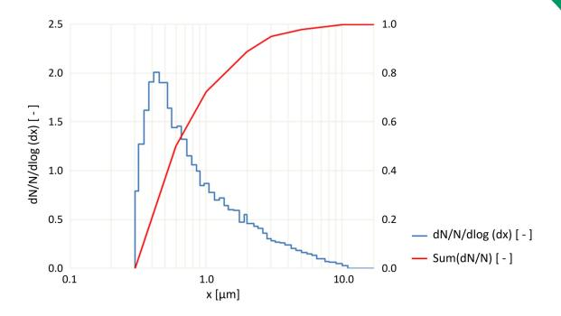
Fig. 2: Particle size distribution with the welas® digital 2000
