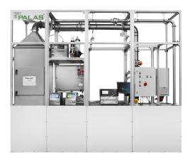
To reliably determine the quality and efficiency of filter elements, it is crucial to test energy consumption (pressure drop), loading, particle separation efficiency, and total penetration.
