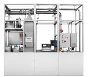
To reliably determine the quality and efficiency of filter elements, it is crucial to test energy consumption (pressure drop), loading, particle separation efficiency, and total penetration.
