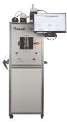
The PMFT 1000 F tests respiratory protection particle filters better than the standards EN 143, ISO 16900-3, and NIOSH 42 CFR 84 with additional accurate analysis of filter mask efficiency for SARS-CoV-2 (size approximately 120 nm to 160 nm). In addition, testing face masks based on EN 149/EN 13274-7 standards is possible. Both total photometric penetration and fractional efficiency are tested, e.g., the efficiency in the whole size range, respectively, the particle size-dependent penetration.
