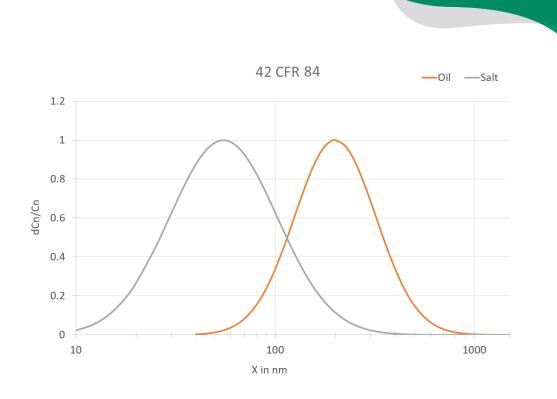
Based on the measurement of the particle penetration via the particle size, the PMFT 1000 F can also be used to consider the tolerances in the particle size distribution according to EN 13274-7 as min. / max. penetration value.
