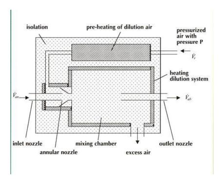
Particle-free air with the volume flow  $V_R$  circulates through an annular passage around the suction nozzle. Thus, according to Bernoulli, a volume flow  $V_{An}$  is generated at the suction nozzle. The volume flow  $V_R$  is heated to the required temperature of the aerosol to be measured using cartridge heaters, such that isothermal conditions prevail. The dilution factor  $V_F$  is calculated according to the following formula:
