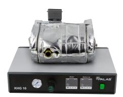
The KHG 10 series of heatable dilution systems builds upon the VKL series ejector principle. In addition to the advantages of the VKL series, the KHG series dilution system is configured to be heatable to 150 °C (optionally up to 200 °C) and is additionally pressure-resistant up to 10 bar pressure. Isothermal and isobaric dilution can therefore be achieved. With the KHG system, both the compressed air supplied and the dilution system are selfheated.
