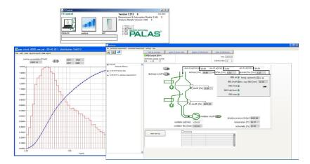
The FTControl software is used for the reliable and economic performance of filter tests and fractional separation efficiency measurements with the welas® digital and Promo®optical aerosol spectrometer.
