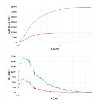
Analysis in table form, including the test conditions Example: Fractional separation efficiency measurement on the MFP 2000
